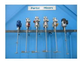
Flamingo Clamp-on Mixers are useful for a wide range of Blending, Dissolving or Dispersing Applications.
